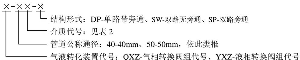
示例：QXZ-40X-DP 40mm 氧气-单路带旁通气相转换阀组
